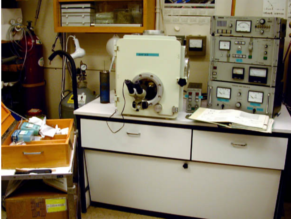
Fig. 1. Balzers BAF 301 FF apparatus similar to the one used in this study. Vacuum chamber is seen in the centre where specimens were processed while being observed with binocular microscope. On the left are tanks containing LN2 hooked up to the apparatus. Sample stage was cooled with constant flow of LN2 when the specimens of tissue were fractured and shadowed with Pt/C.
