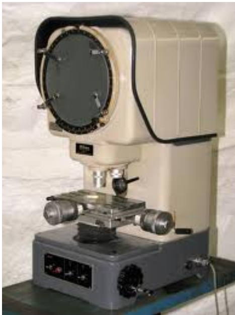
Fig. 6. Nikon projection microscope 6C-2, similar to the one used in this study.
